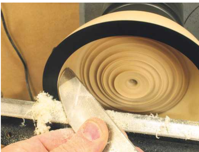
▲ Pic.6 The negative-rake will allow you to present the scraper horizontally. If there's not a downwards angle on the top, then you must present the tool trailing, i.e. with the handle higher than the cutting edge
